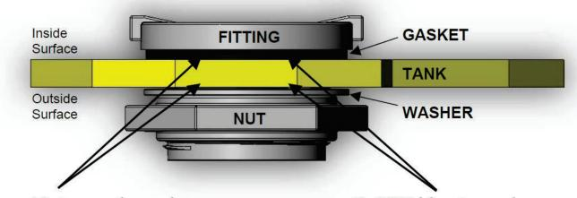
Must remove burr and any shavings on tank surface to allow gasket to seal properly  Do NOT deburr too much material around opening – only remove lip from saw cut, do not carve extra material out
